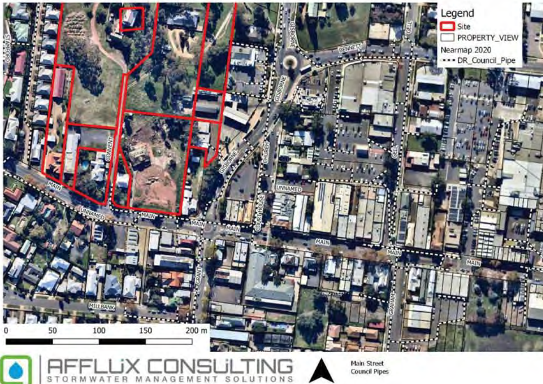
Figure 3 Council Pipes in vicinity of site
