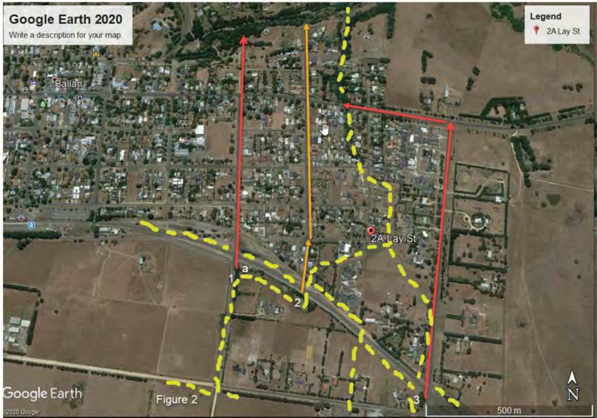
Figure 2. South-east Ballan showing existing drainage patters (yellow line), a). area where water congregates at the intersection of Windle Street and the Railway. 1, 2, and 3 – lines representing suggested changes to drainage.
