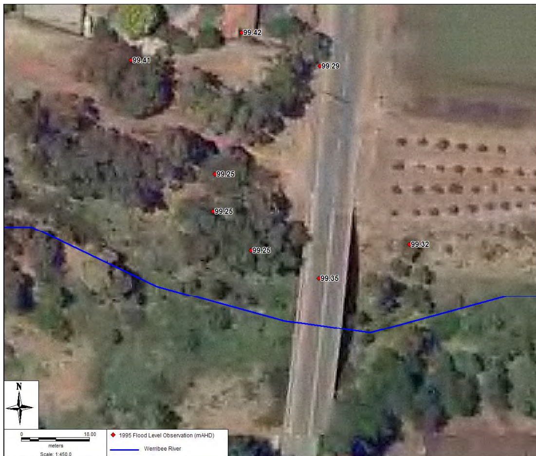
Figure 7-2 Observed Flood Levels near the Fiskin St Bridge – Levels Increasing from downstream to upstream
