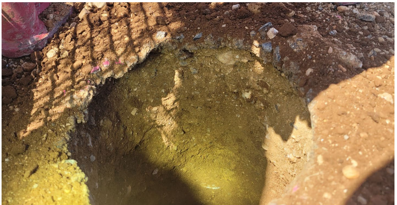
Image 16 – Sprayed seal and pavement gravel in BH03.
