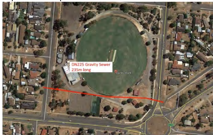
Map 4. The gravity sewer that runs east west across the south end of the Reserve
